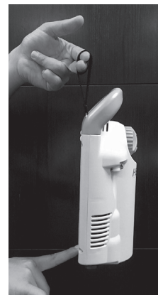
Checking the H300/H850 contents indicator
