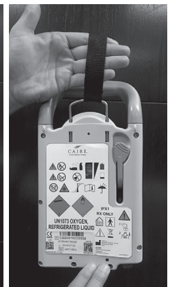
Checking the H300/H850 contents indicator
