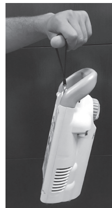
Checking the H300/H850 contents indicator
