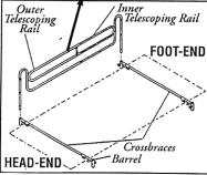
WARNING: To prevent damage to levers and motors of articulating beds, make certain that when the foot and head-ends are raised that the telescoping length of the bed rail is not less than 47 inches. Otherwise the bed rail has bottomed-out and will bind the drive mechanism of the bed. Fither the bed rail or the bed will be damaged.
